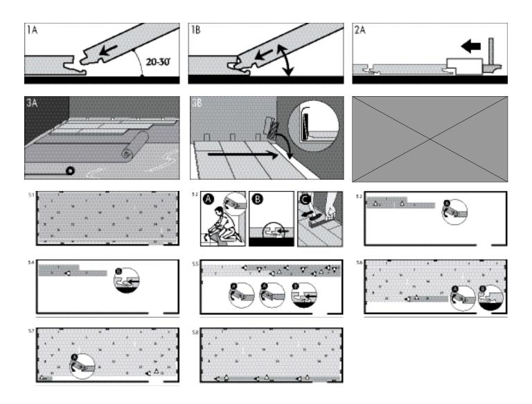
Work out the trims to be installed as some trims are easier to install prior to the flooring. This will be dependent on the direction of the trim to the flooring and the type of trim to be installed.
