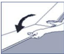
Fig 2. Second plank, first row tilt angle & place this plank gently and tight to the short end of the first one. Angle short end into place. Lengthways tap maybe required to secure tightly. Please make sure both long edges and short ends are tight with no visible gaps.
