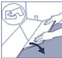
Fig 3. Tilt / Angle the plank down. During the angle process make sure the planks are tight against each other. Afterwards press down or slightly tap down at the short end or long edge of the installed plank till its flat. No major force is or required, use a tapping block or piece of softwood to avoid edge damage.
